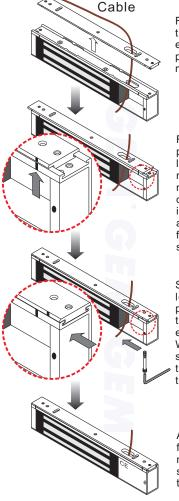
Fasten the mounting plate on the site then install electromagnet lock with power lead cable through mounting plate slot hole.
